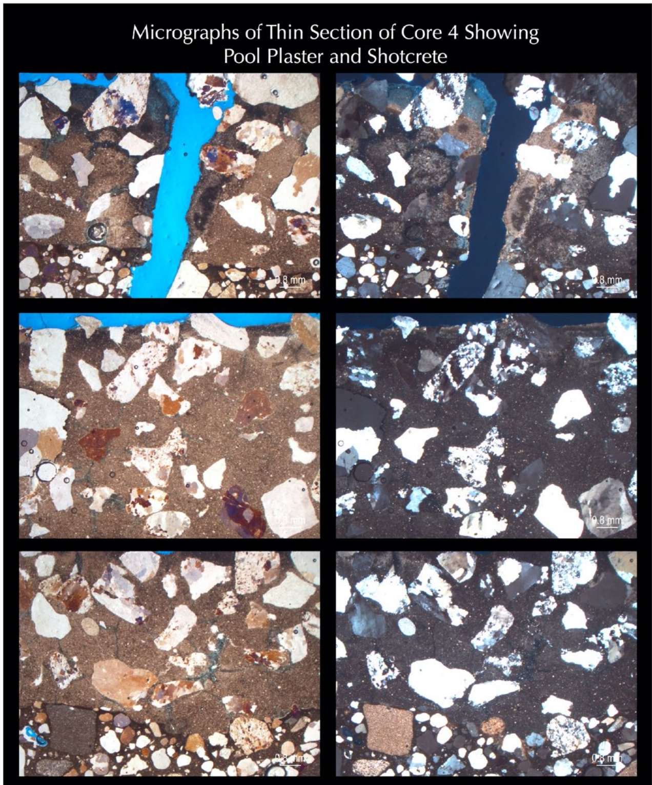
Figure 69: Micrographs of thin section of Core 4 showing: (a) a thin altered zone from pool water interaction on the dense pool plaster having many well-graded, well-distributed sub-rounded to angular (crushed) variably strained siliceous sand filler (2-3 mm size) in dense white cement paste, (b) absence of thin dark brown paste of leveling coat found in three other cores, and (c) the main shotcrete body having crushed limestone and dolomitic limestone aggregate particles, natural siliceous sand aggregate, and interstitial paste with many coarse entrapped air voids. Images were taken in plane (PPL, left) and corresponding cross (XPL, right) polarized light modes respectively, in a stereozoom microscope.
