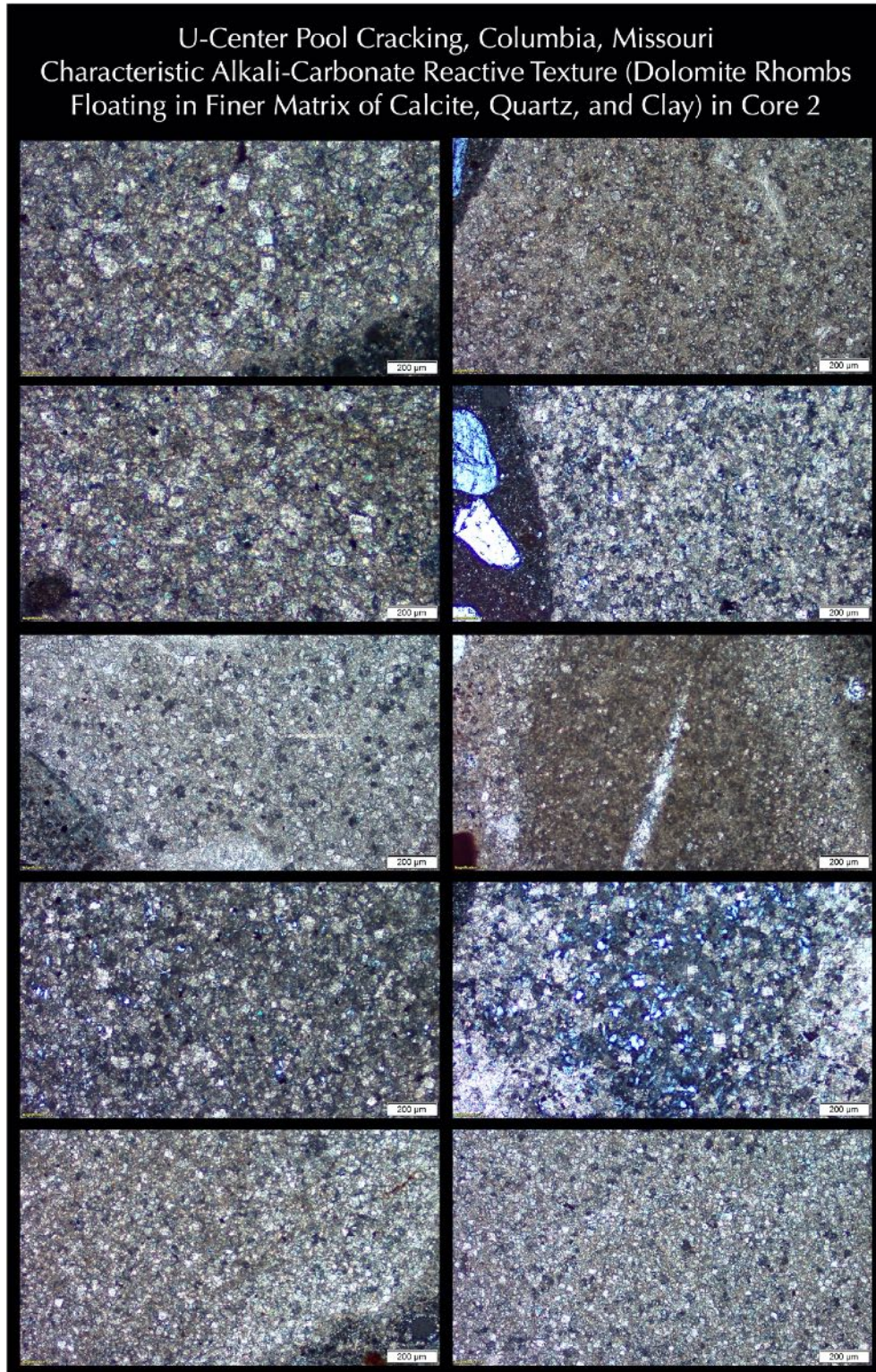
Figure 62: Micrographs of thin section of Core 2 showing characteristic texture of alkali-carbonate reactive (ACR) rocks in shotcrete in having dolomite rhombs floating in finer-grained matrix of calcite, quartz, and clay.
