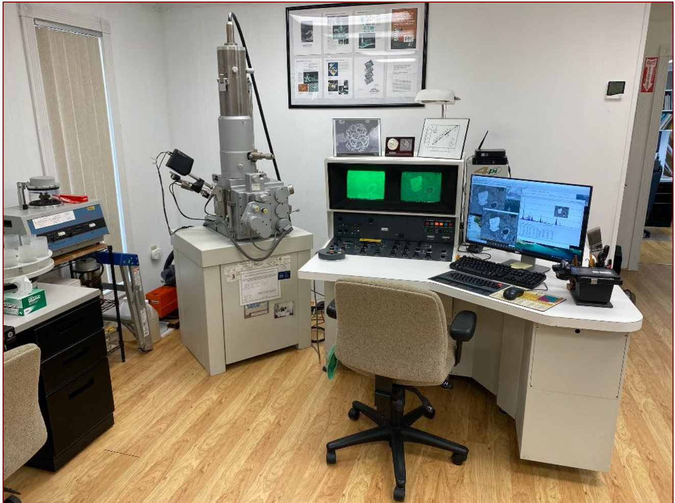
Figure 20: CamScan Series 2 scanning electron microscope used for examination of thin sections of cores for binder compositions of plaster and shotcrete.
