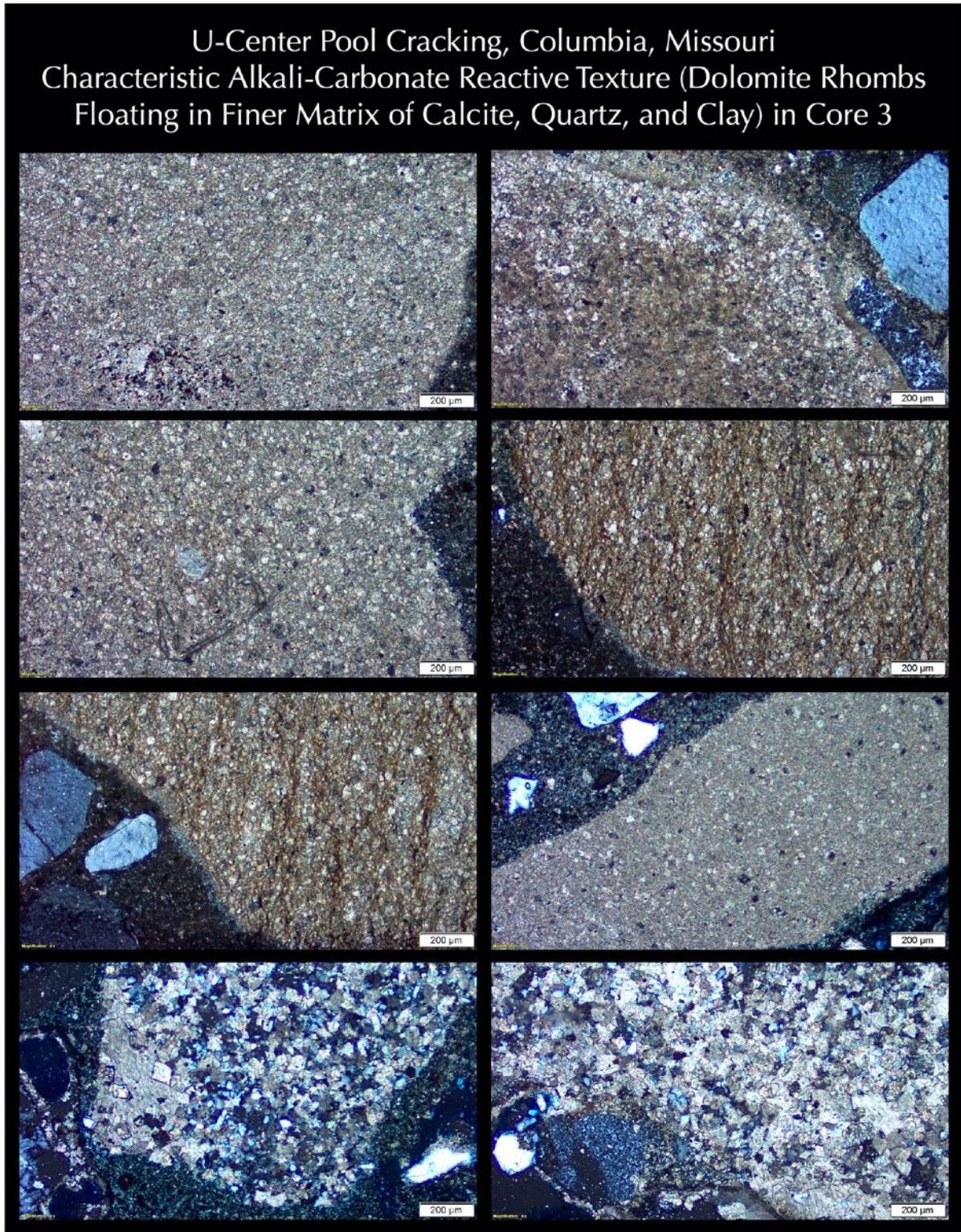
Figure 67: Micrographs of thin section of Core 3 showing characteristic texture of alkali-carbonate reactive (ACR) rocks in shotcrete in having dolomite rhombs floating in finer-grained matrix of calcite, quartz, and clay.
