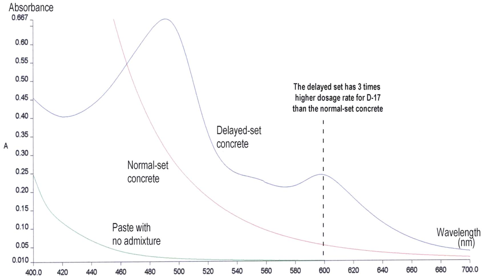
**Figure 5:** UV-Visible spectrophotometer scan of (a) a control paste sample (cement plus fly ash plus water at a 0.50 water-cementitious materials ratio) with no admixture (green); (b) the normal-set concrete sample (red line); and (c) the delayed set concrete sample (blue line). The delayed set concrete clearly shows a significantly higher dosage rate of set retarder (D-17) around the 595 nm region (shown in dashed line).
