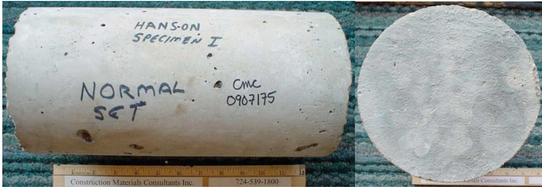
**Figure 1:** Shown are the side and top end of the cylinder for normal set concrete.
