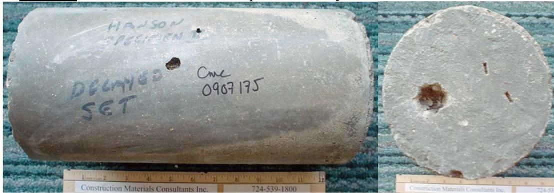
**Figure 2:** Shown are the side and top end of the cylinder for delayed set concrete.
