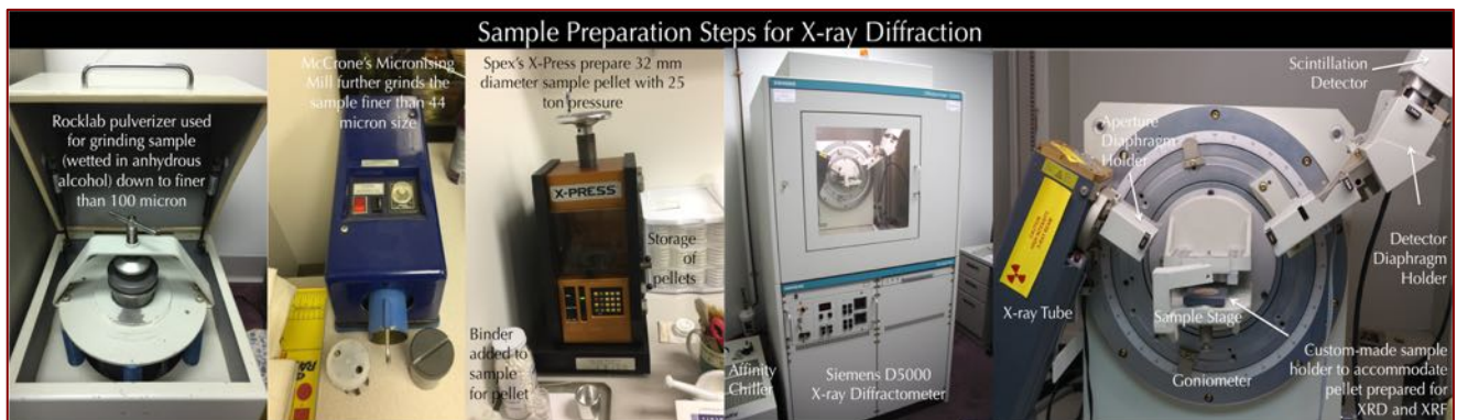
Figure 4: XRD: Siemens D5000 X-ray diffractometer and MDI Jade search/match software used for determination of mineralogical compositions of extracted concrete aggregates. Left to right: Rocklab pulverizer for initial grinding of aggregate with anhydrous alcohol; McCrone micronizing mill for final grinding; Spex 25-ton press for pellet preparation; Siemens D5000 X-ray diffractometer; and custom-made sample holder to place a 32-mm diameter pellet on sample stage.
