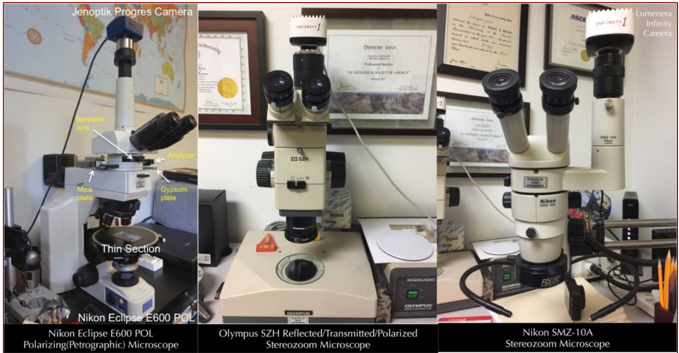
Figure 3: Optical Microscopy: Left - A Nikon Eclipse E600 POL polarizing (petrographic) microscope at left with reflected, transmitted, polarized-light, and fluorescent-light capabilities; Middle – An Olympus SZH reflected/transmitted/polarized-light Stereozoom microscope; and Right – A Nikon SMZ-10A Stereozoom microscope. All microscopes are equipped with Jenoptik Gryphax and Lumenera Infinity digital cameras.
