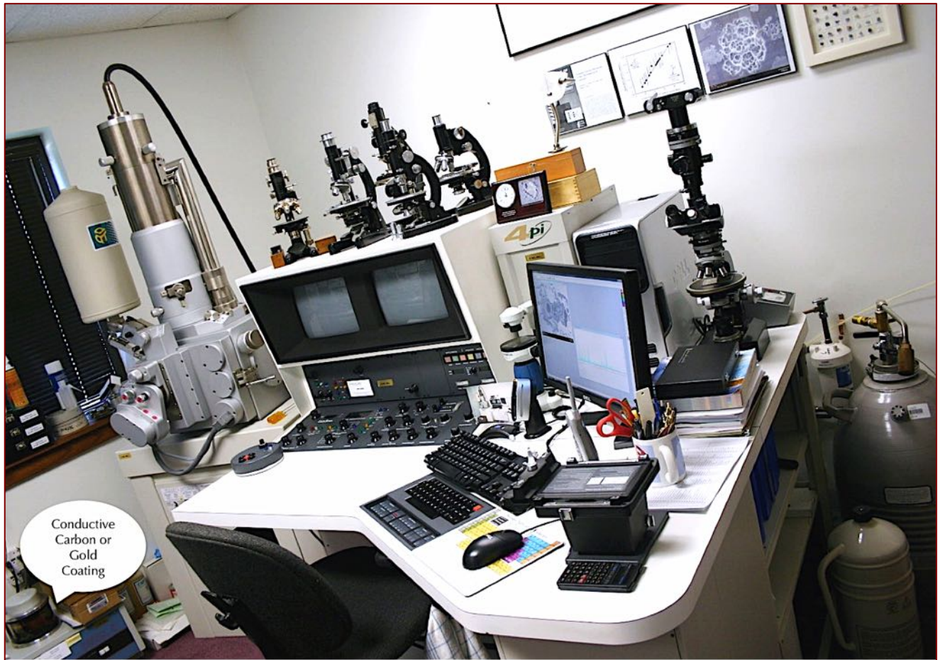
Figure 5: SEM-EDS: Cambridge CamScan Series II Scanning Electron Microscope and 4Pi Revolution software, backscatter detector, secondary electron detector, and energy-dispersive X-ray fluorescence spectrometer used for microstructural and microchemical analyses of concretes and aggregates.
