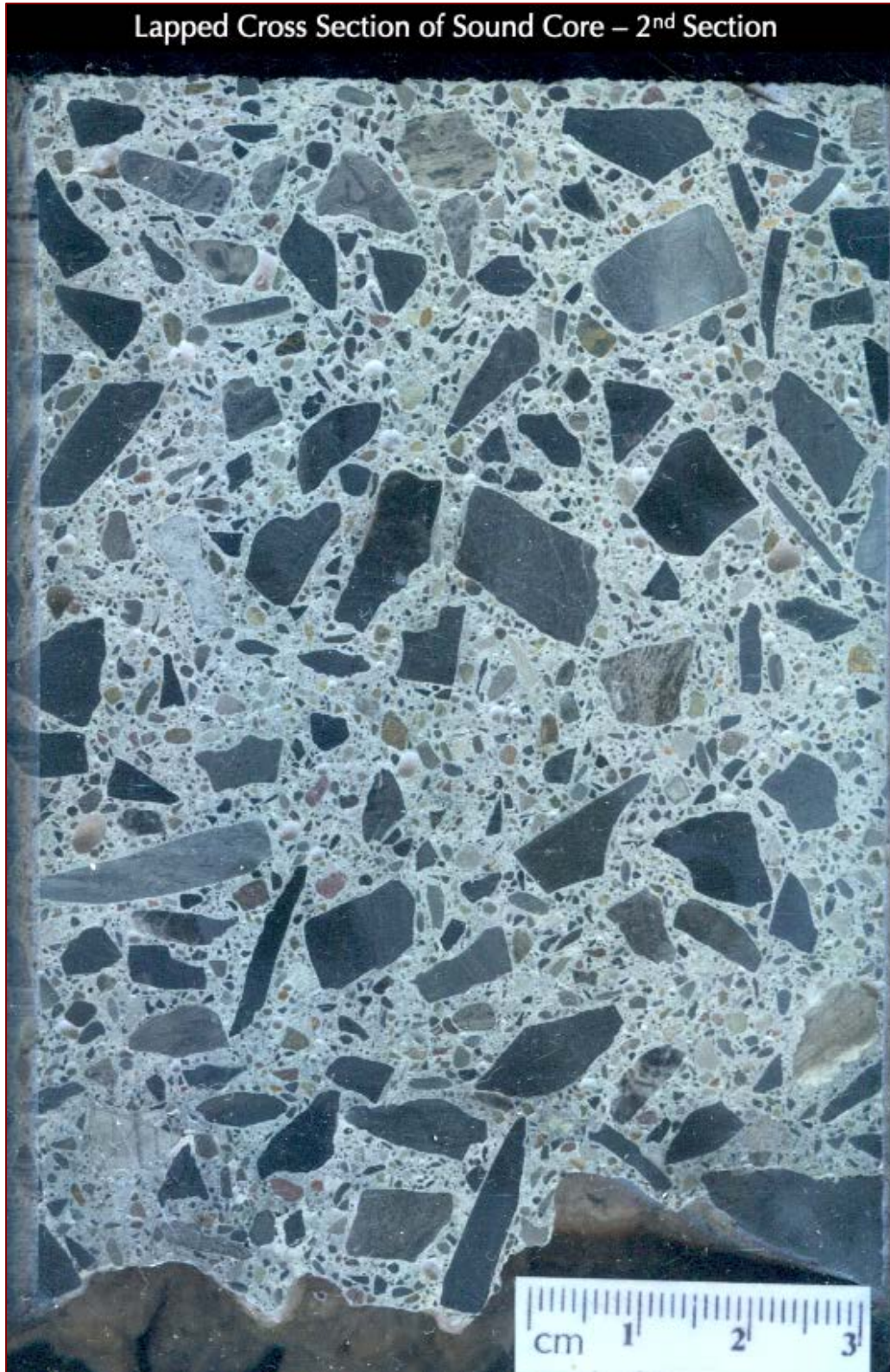
Figure 8: A second lapped cross section of the core from sound area of driveway showing:
