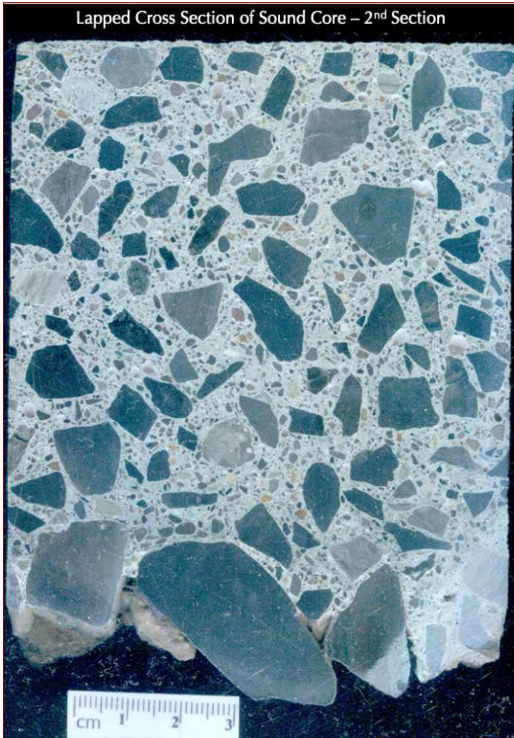
Figure 7: Lapped cross section of the core from sound area of driveway showing:
