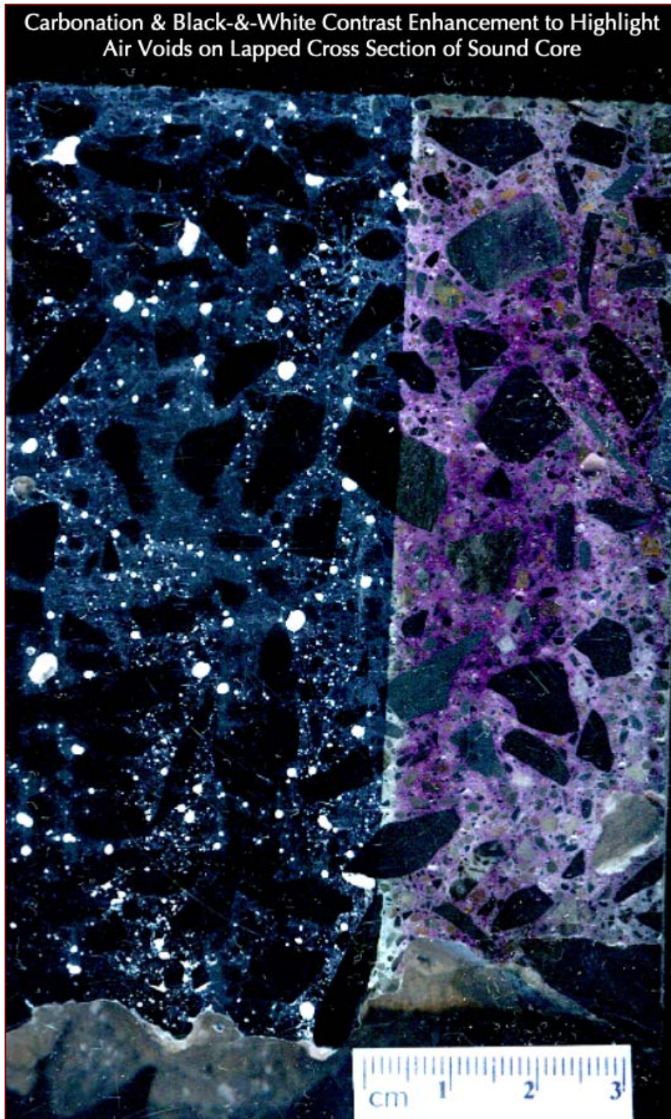
Figure 11: The lapped section of the sound core shown in Figure 8 but after:
