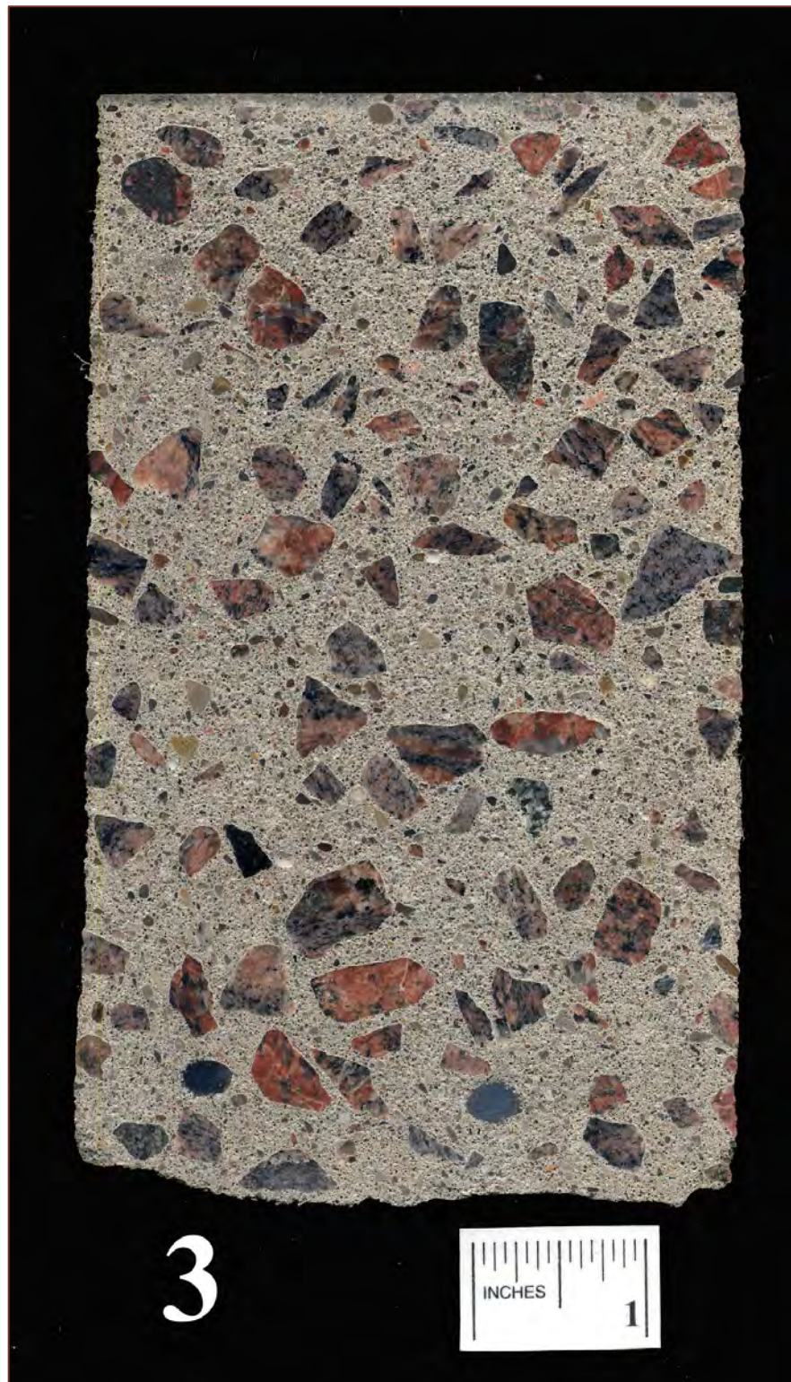
Figure A2: Lapped cross section of Core No. 3 showing: (a) the good grading and well-distribution of the aggregate particles; (b) the densified top surface region; and (c) the moderately dense nature of the interior concrete. Notice a lifting appearance of crushed granite coarse aggregate particles due to frothy texture of the mortar fraction from excessive air entrainment. Also notice the densified surface skin at the top 1/8 in. from trowel finishing.
